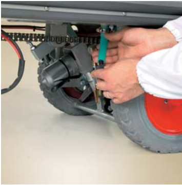
Discharge outlet for any residual fluid of the battery compartment
