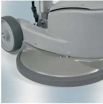
Disc head assembly made of 3 mm thick stamped steel with corrosion-resistant treatments: cataphoresis and epoxy powder painting
