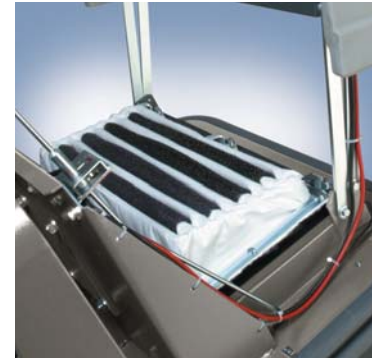
For fine dust, a textile filter (optional) is also available
