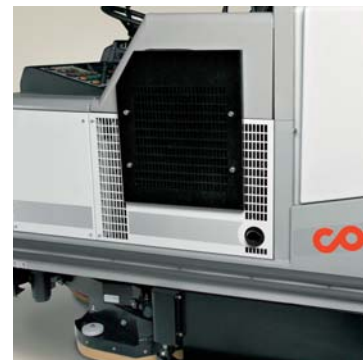
C130 Diesel - Radiator with blowing fan
